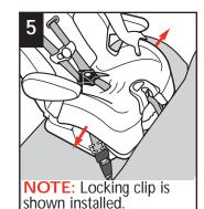
With weakest hand at belt path, tilt and push the child restraint forward and back, and from side to side. If the seat belts do not loosen, your child restraint should be secure.
